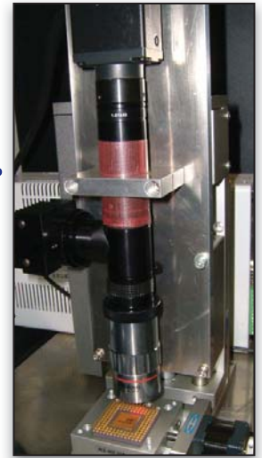
Navitar Ultra Precise Eye inspecting PCB components.
