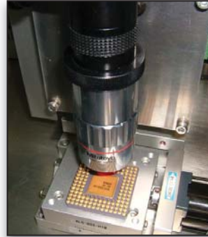
Navitar Ultra Precise Eye inspecting PCB components.
